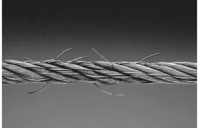
Cable With Broken Wires
